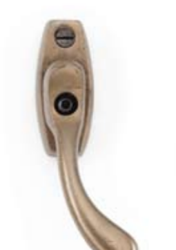
471 Espag. Fastener (lockable) 42mm screw centres, 7mm spindle (handed – right hand shown)
